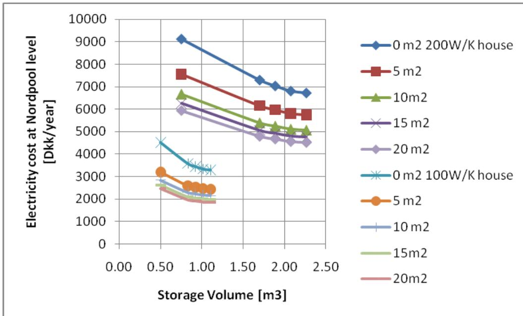
**Figure 4: Raw electricity cost at Nordpool level [4] for differently sized solar combi systems.** Results for two houses, one old and one modern are shown. The 0 m<sup>2</sup> and smallest tank size, indicates the annual electricity cost without solar and only a small effect of smart control.
