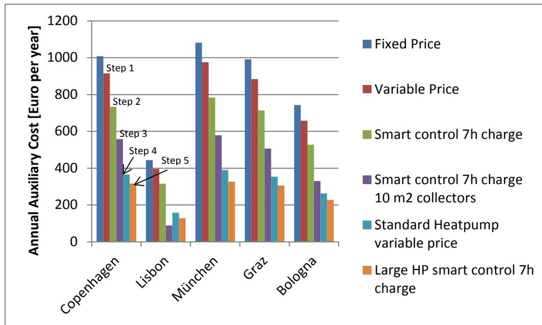
**Figure 5: Annual purchased net energy cost comparison for an old house, at five locations in Europe.** Five different options for smart control and energy saving measures by solar collectors or heat pumps are compared to the cost in a normal house with fixed electricity price all year. The cost per kWh is according to the Nordpool [4] level. No taxes or levies are included.
