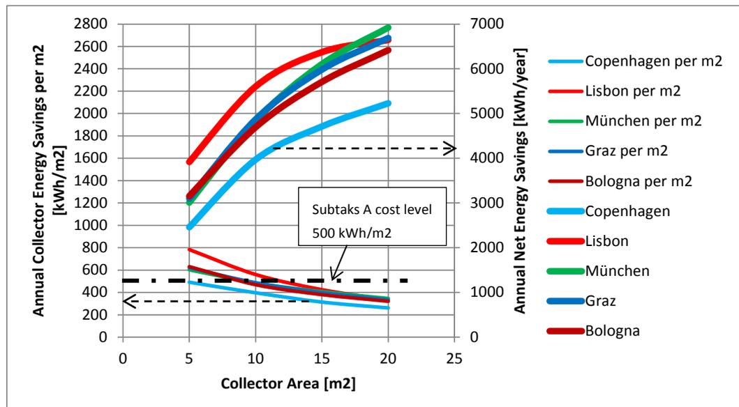
Figure 6: Energy savings by adding solar collectors to an old house (200 W/K)
